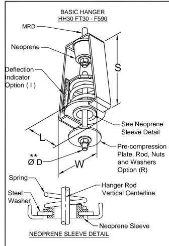
Type HH30 is used where uncertain alignment is anticipated during installation. At rated load the hanger rod will operated to a full 15° tilt in any direction from vertical centerline.
